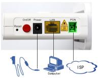
After the cables are properly connected, press down the power switch on the side panel. When the power indicator on the front panel becomes solid on while the other indicators are normal, the services that the operator provides are available
